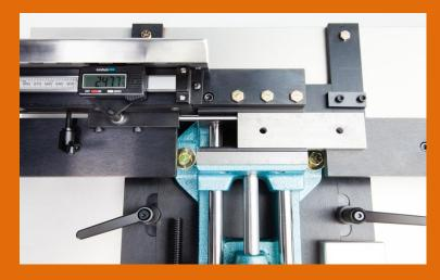
ABOVE IS A SAMPLE PART IN THE POSITIONER. NOTICE THE X-AXIS DIGITAL SCALE IS SHOWN WITH HINGED COVER LIFTED.
